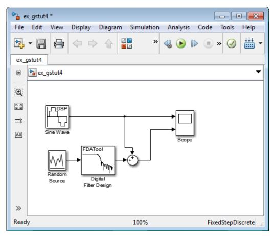
Run your model and view the results in the Scope window. This window shows the original input signal and the signal with low frequency noise added to it.
